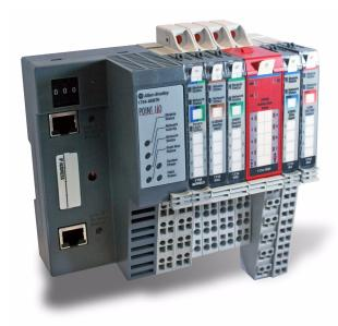
Each POINT I/O module mounts adjacent to the network adapter or another I/O module and removable terminal block (RTB) to connect all field-side wiring. The RTBs are part of the terminal base assembly. They are not included with the I/O modules and must be ordered separately.
